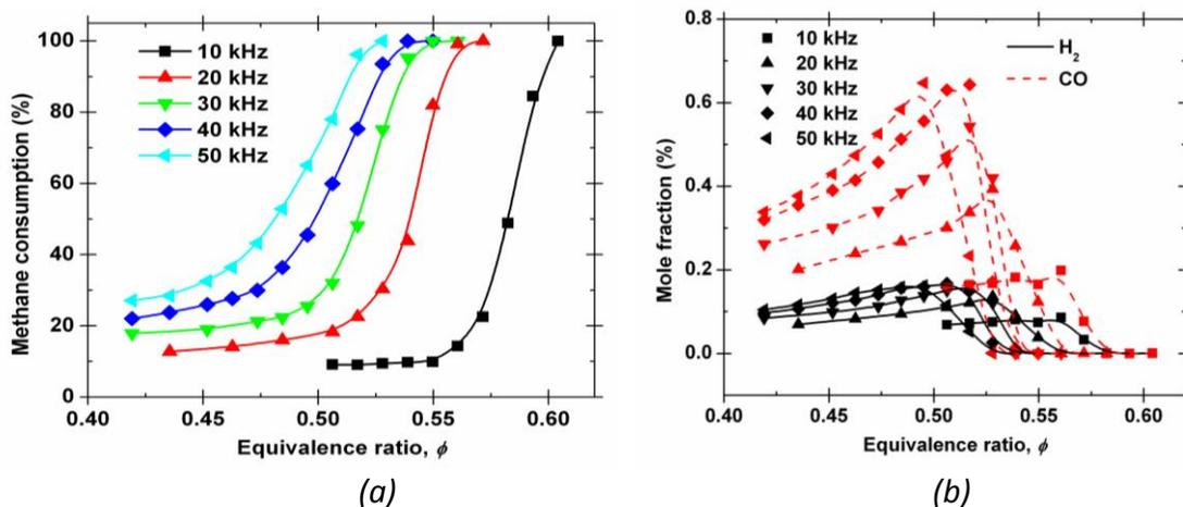
Fig. 1. (a) Methane consumption and (b)  $H_2$  and CO mole fractions as a function of discharge repetition rate (constant average power) at an 11 mm fixed downstream location from the discharge.
