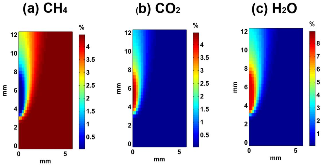
Fig. 4. Quasi-steady state spatial distribution of (a)  $\text{CH}_4$ , (b)  $\text{CO}_2$ , and (c)  $\text{H}_2\text{O}$  for a discharge repetition rate of 10 kHz and a 9 ns pulse width. The discharge is located between 3 and 4 mm in axial location and is 1 mm in radial dimension.
