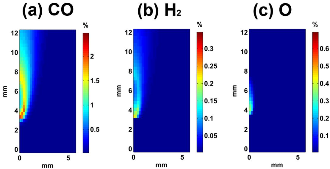
Fig. 5. Quasi-steady state spatial distribution of (a)  $\text{CO}$ , (b)  $\text{H}_2$ , and (c)  $\text{O}$ , for a discharge repetition rate of 10 kHz and a 9 ns pulse width.
