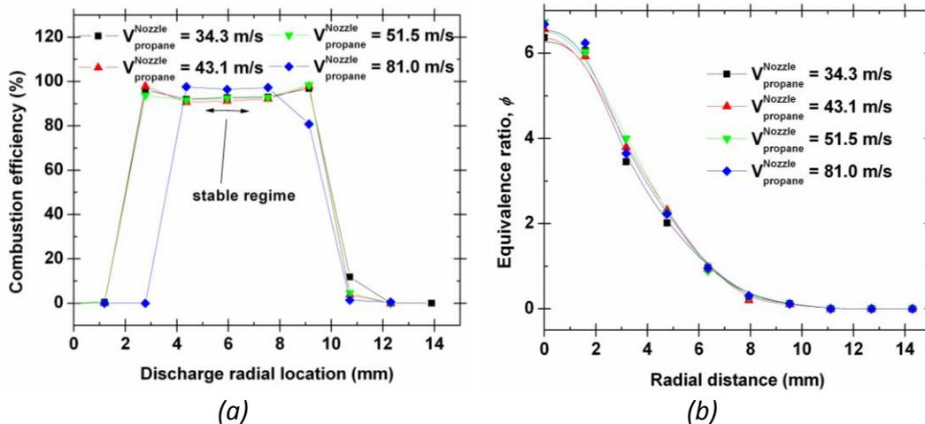
Fig. 3. (a) Propane jet combustion efficiencies at a fixed axial downstream location given radial discharge locations and (b) the corresponding equivalence ratios at the discharge locations.
