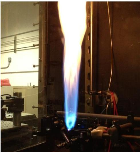
*Fig. 2. Photograph of discharge-stabilized propane-jet flame. The discharge is located where  $\phi \approx 1.27$ , the jet speed is 43.1 m/s, and air coflow speed is 0.8 m/s.*
