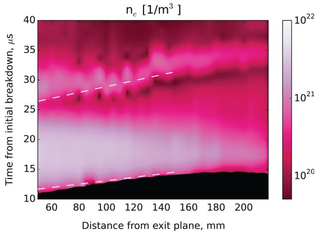
FIG. 3 (color online). Contours of free electron density in  $z$ - $t$  space, shown as a function of distance from the accelerator exit plane in the axial direction and time from initial breakdown following primary gas injection. Regions of space and time in which the QLP equation system did not converge (i.e., no currents were being collected from the plasma) are represented by the black area in the lower portion of the figure. The leading edge contours of both waves are highlighted in Fig. 5.
