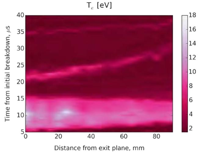
Figure 3: Contour of the plasma / electron temperature along the axis as a function of time. Structure of the temperature contour is less pronounced, particularly for the second and third ejections. An overall mean temperature of  $\sim 10\text{-}12 \text{ eV}$  is observed in the initial deflagration jet, and the effective pulse width experienced by the target is determined based on this contour to be  $\sim 10 \mu\text{s}$ .
