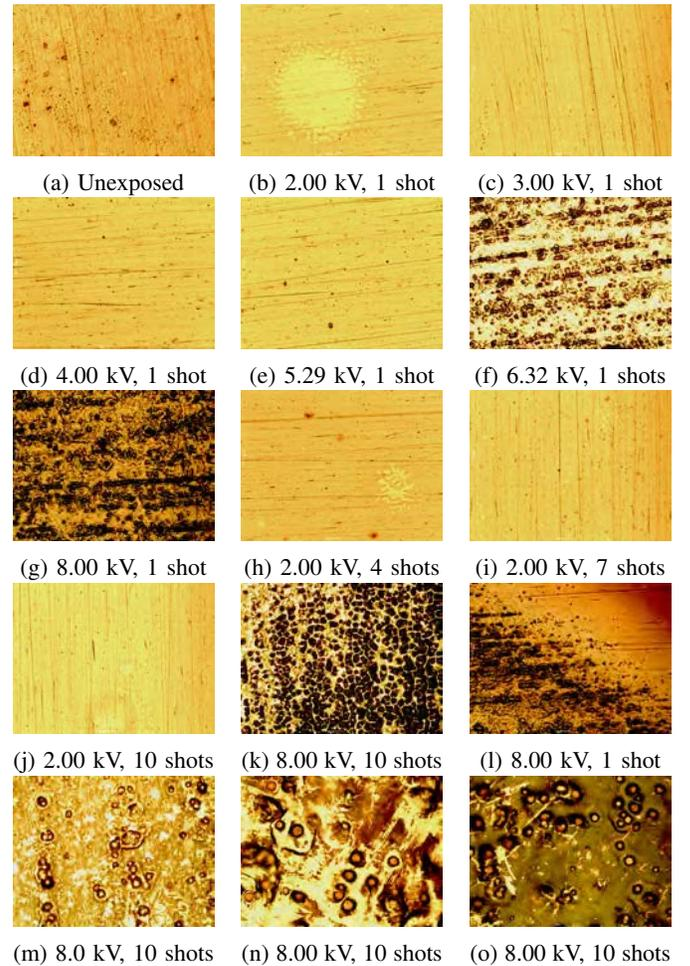
Figure 4: Compilation of optical micrographs corresponding to all the tested conditions in the witness plate study. Subfigures (a)-(l) correspond to the same magnification (scale bar visible), whereas subfigures (m)-(o) are images taken at a higher magnification.
