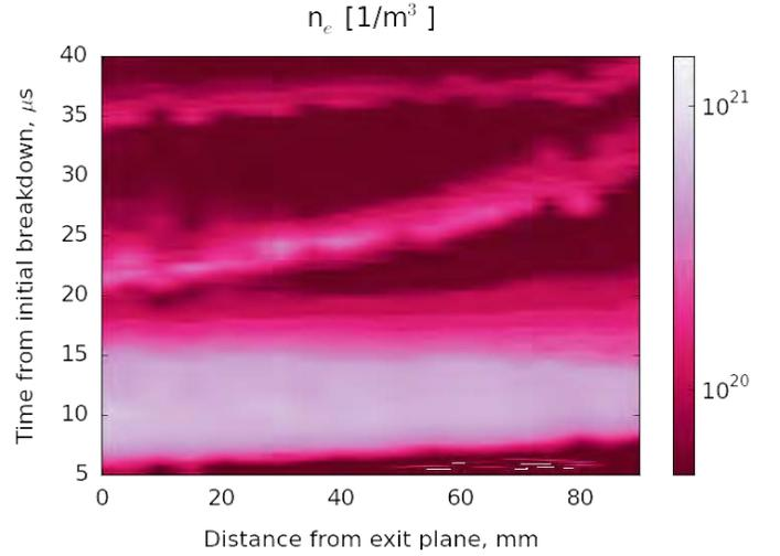
Figure 2: Contour of the plasma density along the axis as a function of time. Three plasma ejections are clearly visible, corresponding to three ringdown oscillations of the driving capacitor bank. Peak densities are of  $10^{21} \text{ m}^{-3}$  are observed in the initial deflagration jet.
