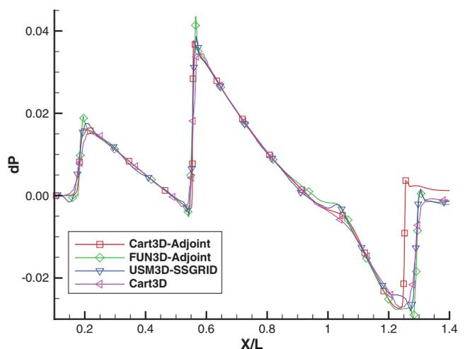
Fig. 27 Nondimensional pressure signature for the delta-wing-body at  $h/l = 2.8$ .
