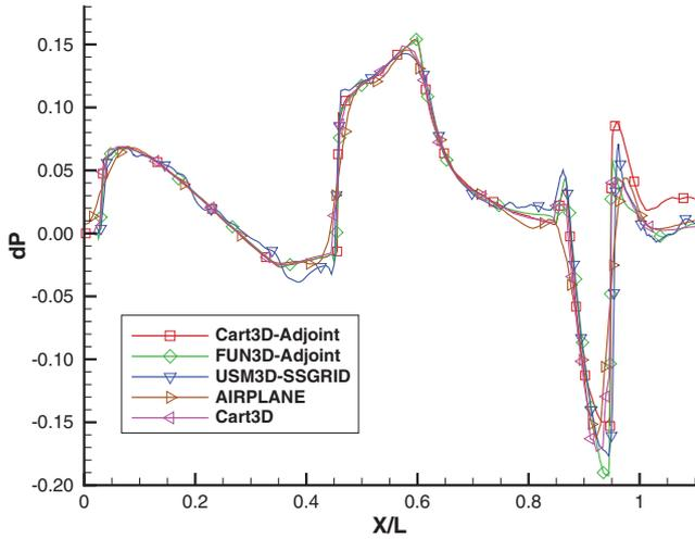
Fig. 22 Nondimensional pressure signature for the delta-wing-body at  $h/l = 0.2$ .
