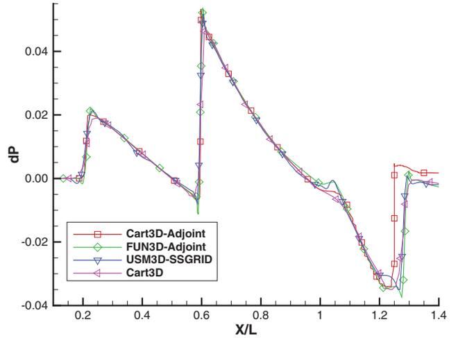
Fig. 26 Nondimensional pressure signature for the delta-wing-body at  $h/l = 2.0$ .
