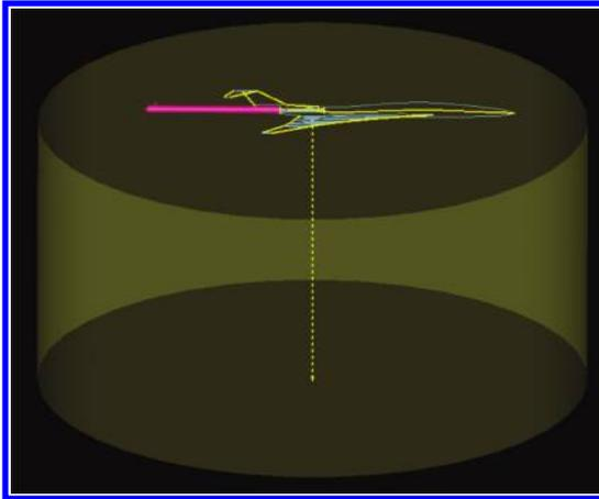
Fig. 11 VGRID line and volume sources for boom analysis, including plume effects.
