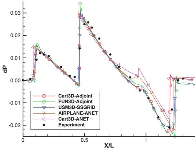
Fig. 28 Nondimensional pressure signature for the delta-wing-body at  $h/l = 3.6$ .
