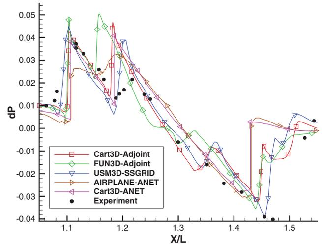
Fig. 31 Center section of the nondimensional pressure signature for the LBWT at  $h/l = 1.167$ .
