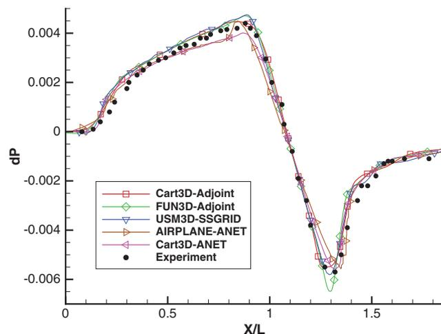
Fig. 15 Nondimensional pressure signature for the cone-cylinder geometry at  $h/l = 10.0$ .
