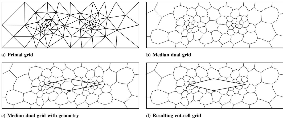
Fig. 8 Cut-cell illustration of a diamond airfoil in 2-D with a simplex background grid.
