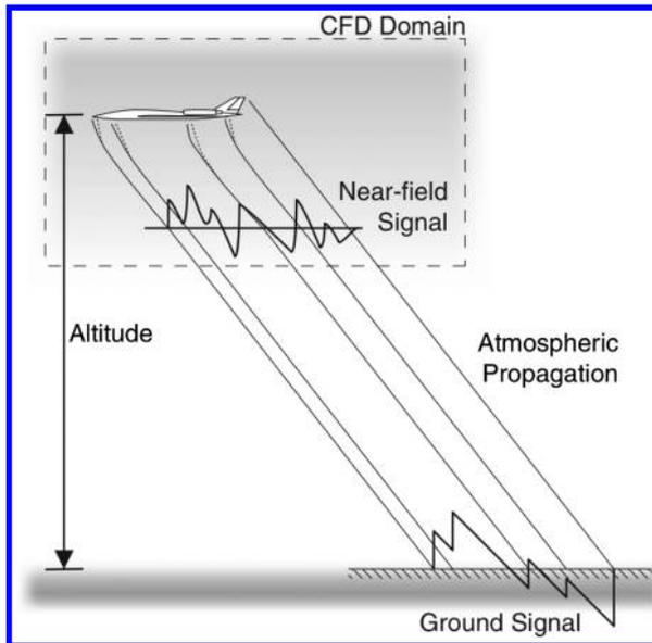
Fig. 1 Sonic-boom signal propagation [6].
