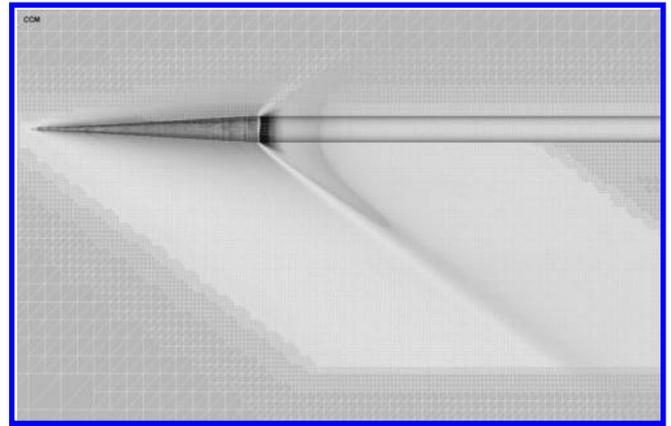
Fig. 5 Symmetry plane grid and pressure coefficient with EASS refinement region for the cone-cylinder configuration, Cart3D aligned to the x axis, Mach 1.68,  $\alpha = 0.0$  deg.
