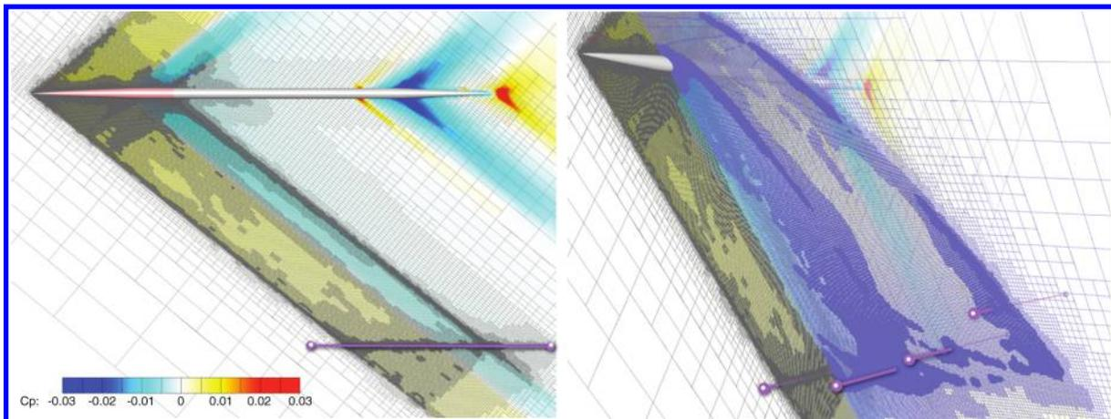
Fig. 7 Cart3D-adjoint mesh (13 million cells) colored with pressure [6]. Adaptation driven by sensors at  $h/l = 1.8$  and  $\varphi = 0, 15, 30$  and  $45$ .
