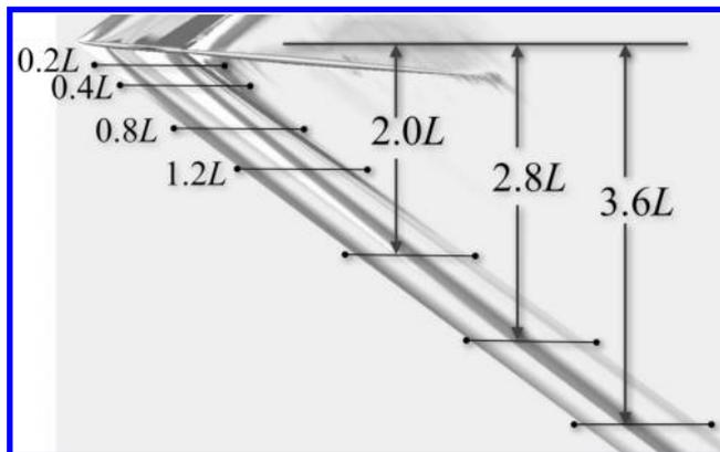
**Fig. 21** Delta-wing-body signature extraction locations.
