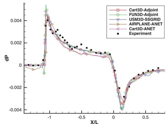
Fig. 17 Nondimensional pressure signature for the parabolic geometry at  $h/l = 10.0$ .
