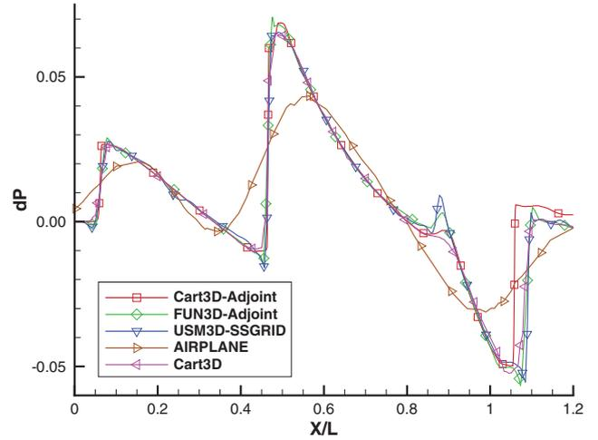
Fig. 25 Nondimensional pressure signature for the delta-wing-body at  $h/l = 1.2$ .
