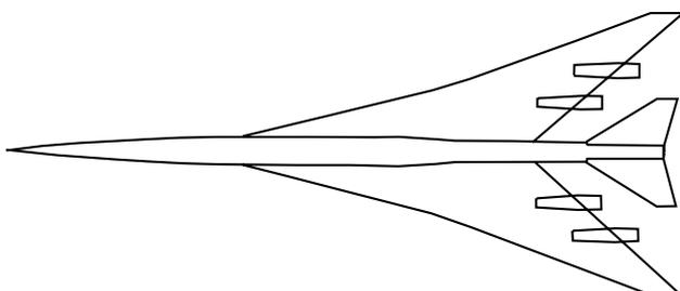
Fig. 29 Planform of the LBWT fuselage, wings, tails, and engines.
