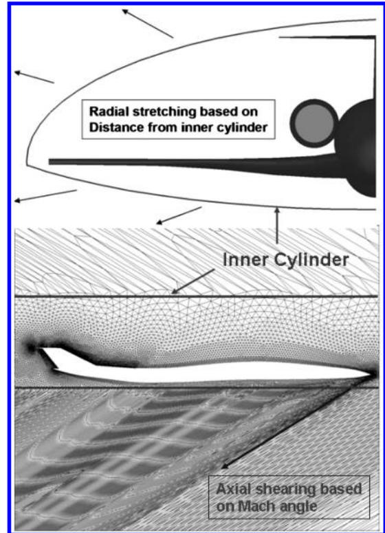
Fig. 13 Grid stretching and shearing controlled by an inner cylinder.
