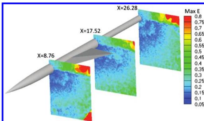
Fig. 4 Delta-wing-body and contours of maximum edge length in an EASS region.
