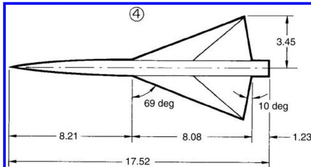
**Fig. 20** Delta-wing-body geometry, in centimeters and degrees [9]. The body length is defined as 17.52 cm.
