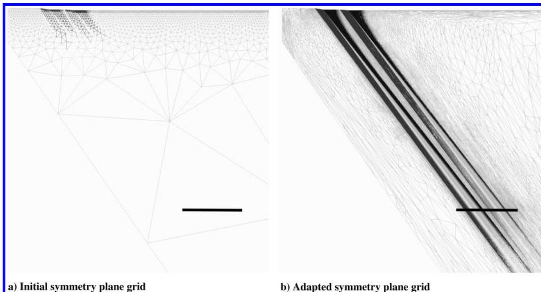
Fig. 9 Symmetry plane grid colored with pressure for an axisymmetric configuration FUN3D-adjoint simulation [45]. The intersection of the sensor surface with the symmetry plane is shown in black.
