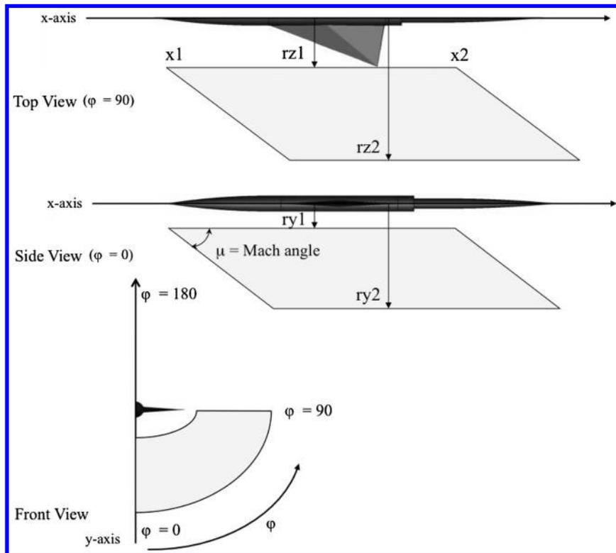
**Fig. 2** Diagram of EASS refinement region parameterization.
