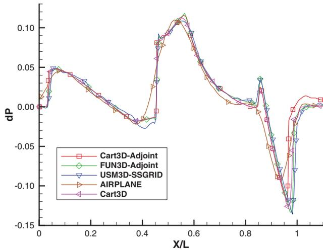
Fig. 23 Nondimensional pressure signature for the delta-wing-body at  $h/l = 0.4$ .
