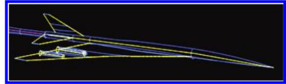
Fig. 10 VGRID line sources (in yellow) automatically generated by AUTOSRC.
