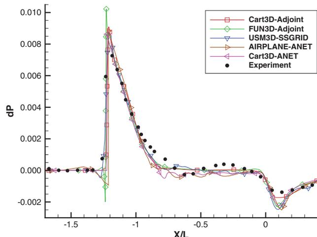
**Fig. 19** Nondimensional pressure signature for the quartic geometry at  $h/l = 10.0$ .
