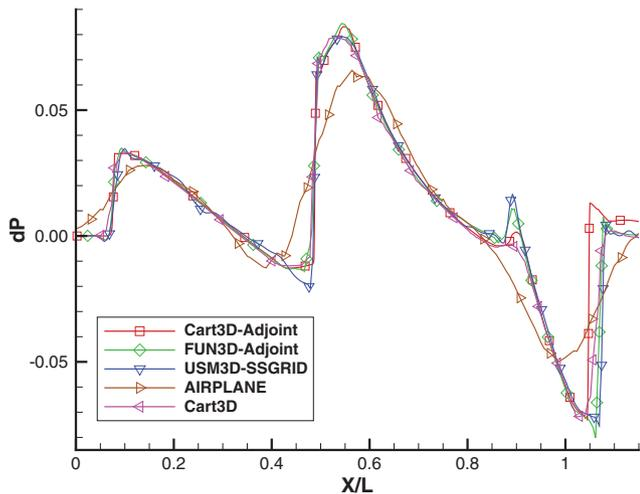
Fig. 24 Nondimensional pressure signature for the delta-wing-body at  $h/l = 0.8$ .
