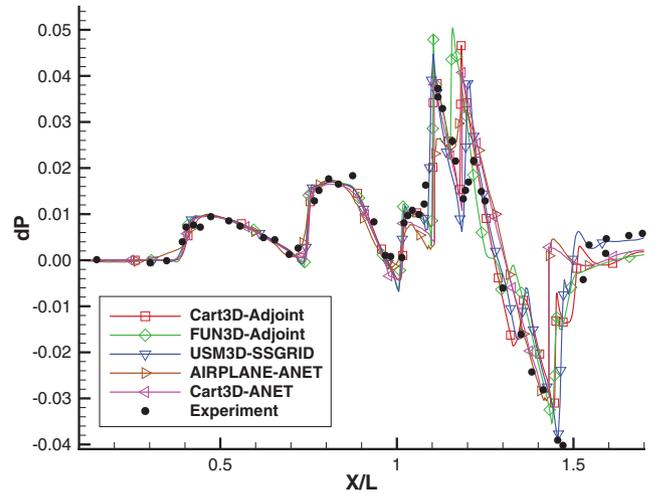
Fig. 30 Entire nondimensional pressure signature for the LBWT at  $h/l = 1.167$ .
