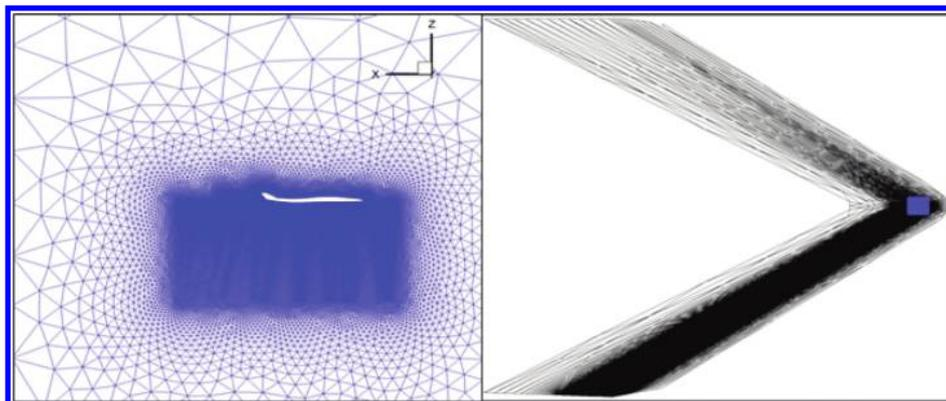
Fig. 12 Original (left) and final stretched/sheared symmetry plane grid from SSGRID.
