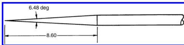
Fig. 14 Cone-cylinder geometry (dimensions in degrees and inches) [7]. The model is defined as the cone.
