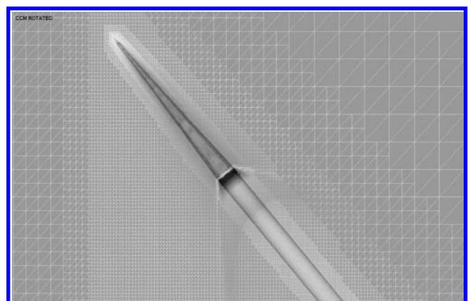
Fig. 6 Symmetry plane grid and pressure coefficient with EASS refinement region for the cone-cylinder configuration, Cart3D aligned to freestream Mach angle, Mach 1.68,  $\alpha = 0.0$  deg.
