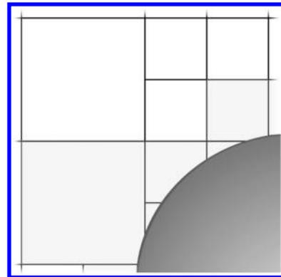
**Fig. 3** Multilevel Cartesian mesh in two-dimensions with a cut-cell boundary.
