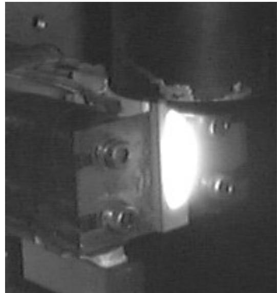
**Figure 5.** Photograph of the linear-geometry open electron-drift Hall discharge while operating.
