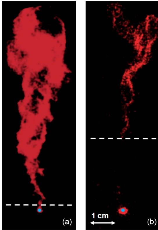
Fig. 2. Instantaneous CH chemiluminescence image: At (a) 300 K and (b) 940 K ambient temperatures. The discharge conditions are 10-kV peak voltage and 50-kHz repetition rate, and the discharges are located in the region identified by blue dots. The flow speeds are (a) 4 and (b) 4.2 m/s. The white dashed lines represent the flame base location.
