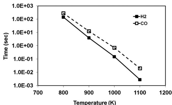
Fig. 4. 90% concentration decay time of H<sub>2</sub> and CO in a postcombustion mixture whose original equivalence ratio is 0.67. Initial concentrations of H<sub>2</sub> and CO are 5000 ppm each. CHEMKIN with GRI MECH 3.0 was used for this simulation.
